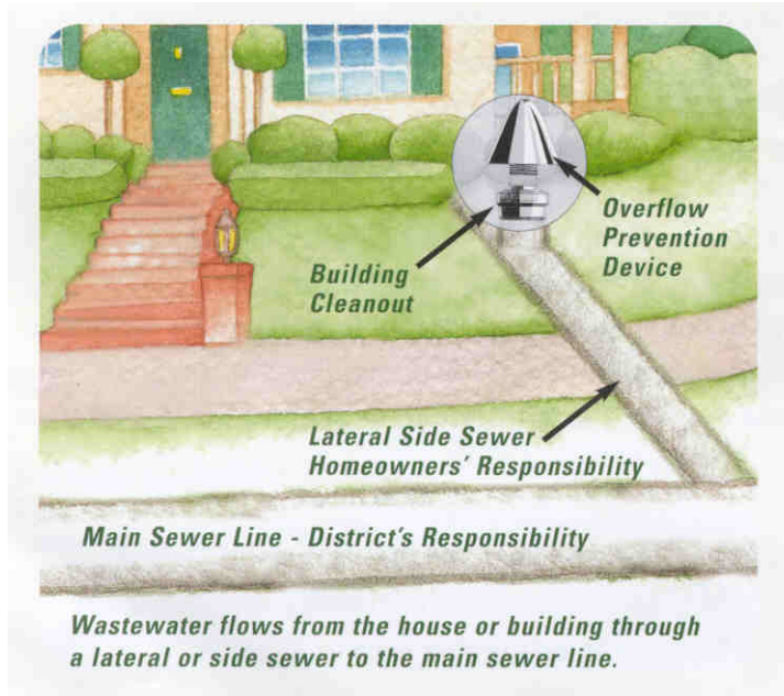
Figure 2 Typical Sanitary Sewer System
